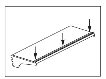
(5) Secure aluminum mounting rail to the front of the existing shelf with provided fasteners.
