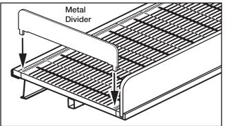
Install first divider starting with the furthest left slots of the FlexRoller shelf.
