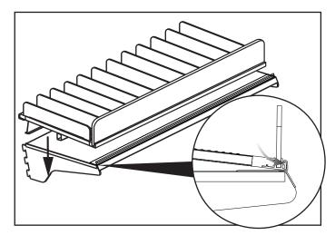
(6) 2 people to lift the FlexRoller and place on existing shelf engaging the FlexRoller with the Aluminum Mounting rail.
